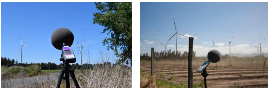
Fig. 5 – Wind shield required for the application of the DS 38 in WTN.
