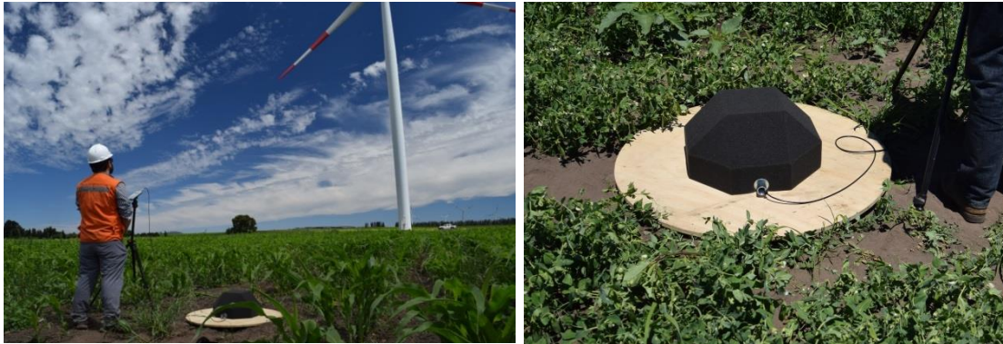
Fig. 9 – Sound power level measurement equipment according to IEC 61400-11.
